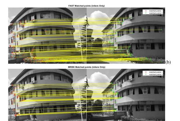
Figure 4.0: Matching of image 1 with image 2 using: (a) SURF (b) FAST (c) BRISK
