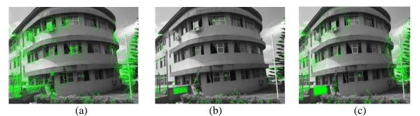
Figure 3.0: Feature detection of image 1 using: (a) SURF (b) FAST (c) BRISK
